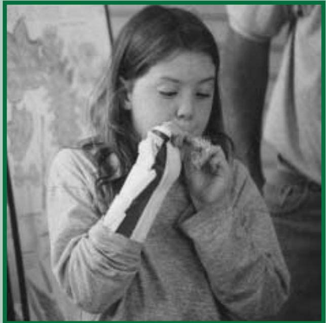
**This student is attempting to blow soap bubbles through a wood dowel. During this lesson, the students learn about the permeability of different types of wood and their cell structure.**
