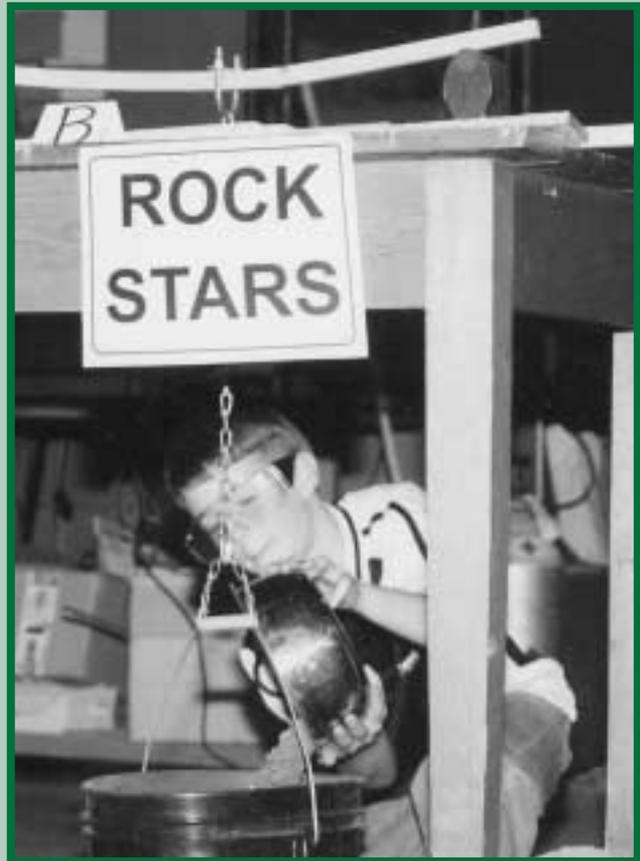
**The strength of sticks of wood in bending is being tested here by loading the bucket that has been suspended from the stick with rocks until the stick breaks. During this lesson, students also discover the influence of growth rings on the strength of wood.**
